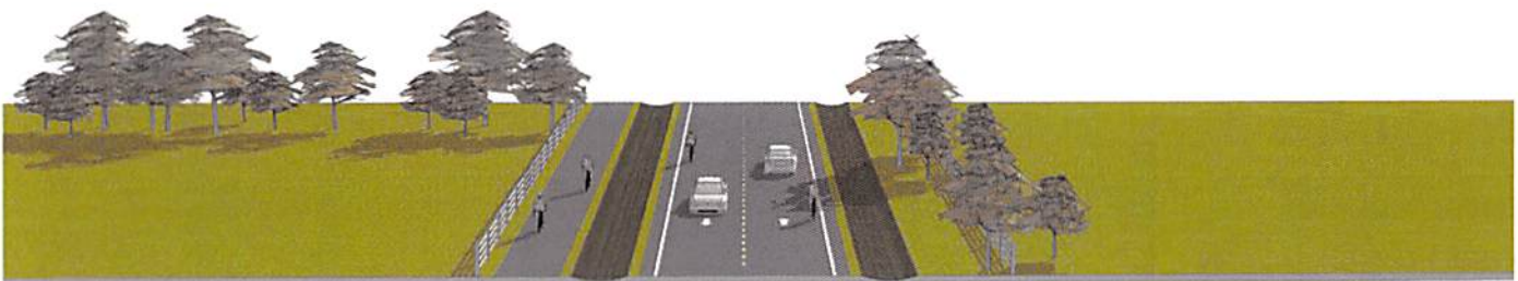
Rural Setback | 8' Leisure Trail | Ditch | 12' | 12' | Rural Streetscape | Rural Setback 2 Travel Lanes (24'-33.5' Total Pavement Width)
