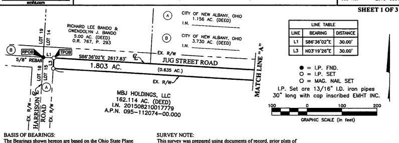
The Bearings shown hereon are based on the Ohio State Plane Coordinate System South Zone as per NAD83 (1986 Adjustment). Said bearings originated from a field traverse which was tied (referenced) to said coordinate system by GPS observations and observations of Franklin County Engineering monuments Frank 80 and Frank 180. The portion of the centerline of Beech Road, having a bearing of North 02° 57' 02" East, is designated the "basis of bearings" for this survey.
