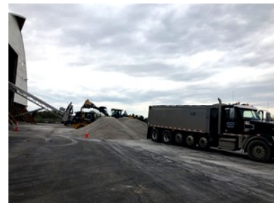
Franklin County material conveyor is used for piling salt in the storage barn.
