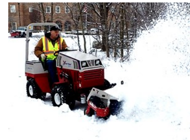
Supervisor Doug Wittman tests out a Ventrac 4500 tractor for trail snow removal.
