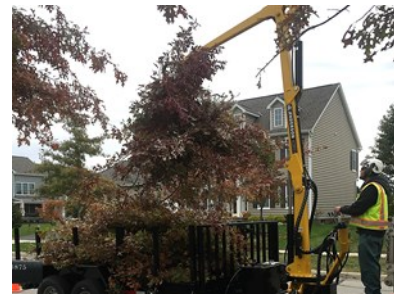
New grapple trailer picks up brush after pruning a pin oak street tree.
