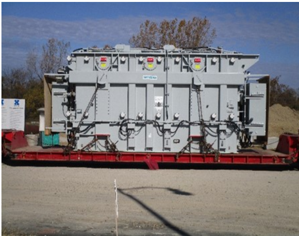
A transformer is carried into the Google site by a Goldhofer trailer
