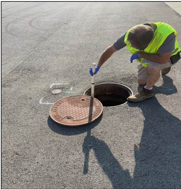
Dave Thatcher measuring and recording Sediment levels for the fleet Garage interceptor
