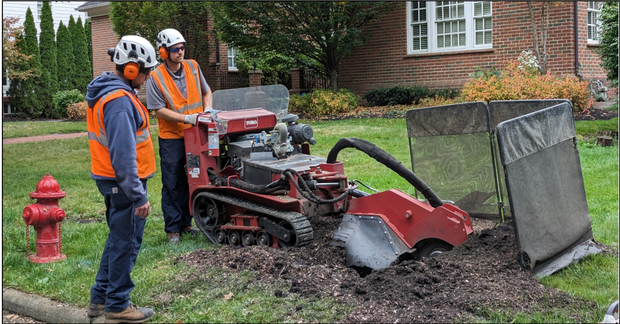
Sam Darnall grinds a stump while Chase Loughman watches for underground obstacles.
