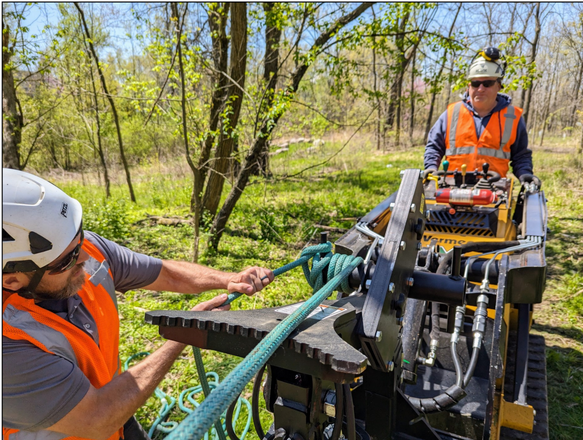
Chase Loughman ties a rope off to the bollard on the new forestry grapple so Mike Cligrow can help direct the fall of a tree at Resch Park
