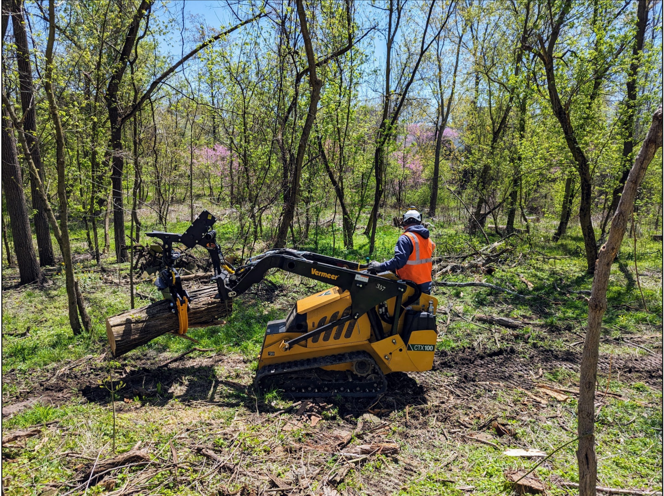
Mike Cligrow transports logs to the chipper using the new forestry grapple
