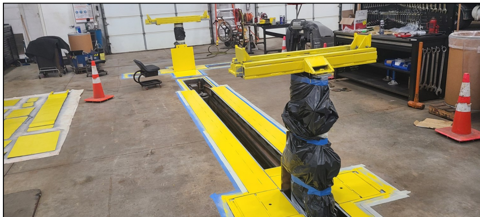
All pieces of the lift after sandblasting, priming and painting completed
