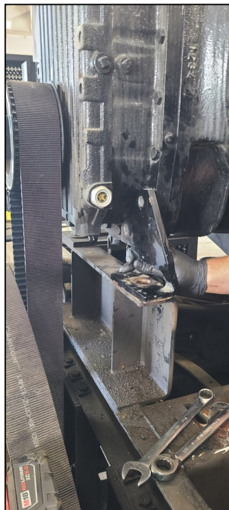
Left: Before fabrication and welding new part to hold new water pump Center and Right: After fabrication and welding completed
