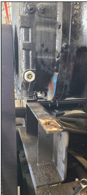
Left: Before fabrication and welding new part to hold new water pump Center and Right: After fabrication and welding completed
