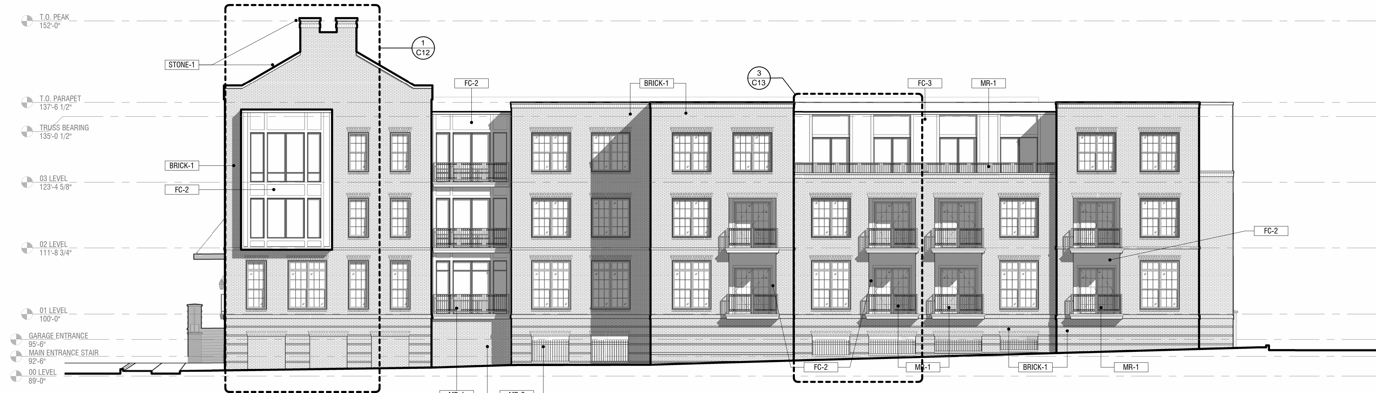
ELEVATION - WEST 2 BUILDING ELEVATION SCALE 3/32" = 1'-0"
