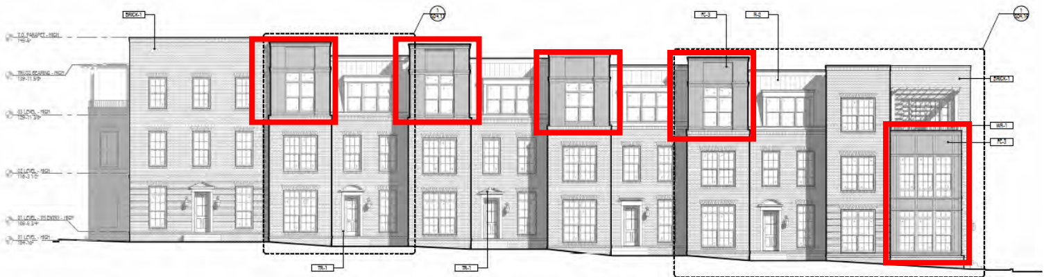
Example of how hardi-board is used throughout the development (shown in red)
