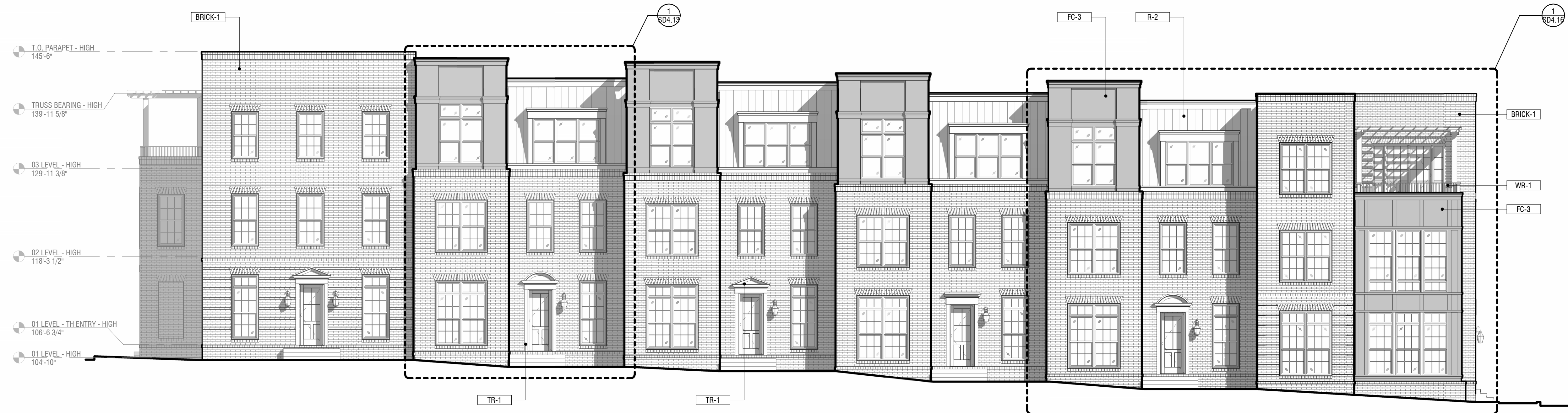
East Elevation - Second Street 1 BUILDING ELEVATION SCALE 1/8" = 1'-0"
