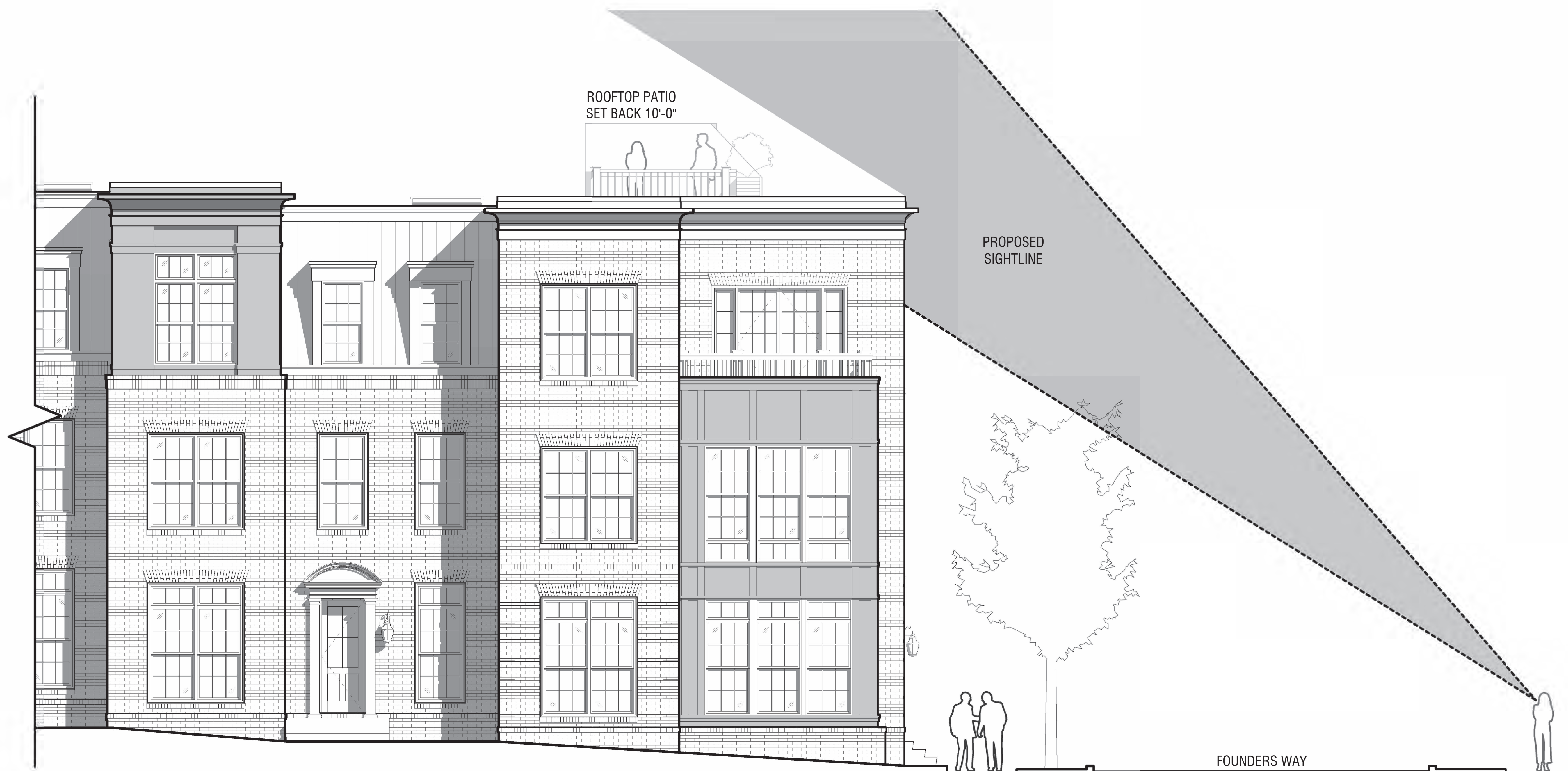
East Elevation_Visibility Study 1 BUILDING ELEVATION SCALE 1/4" = 1'-0"
