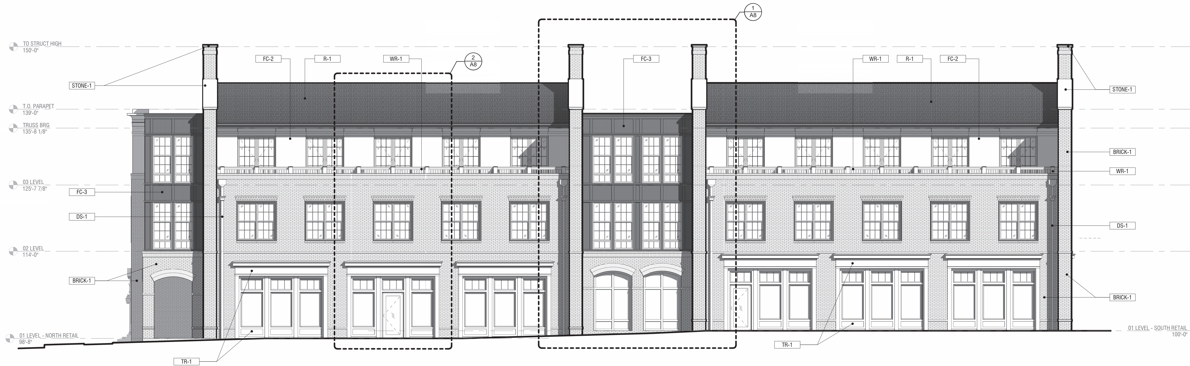
WEST - HIGH STREET 1 BUILDING ELEVATION SCALE 1/8" = 1'-0"
