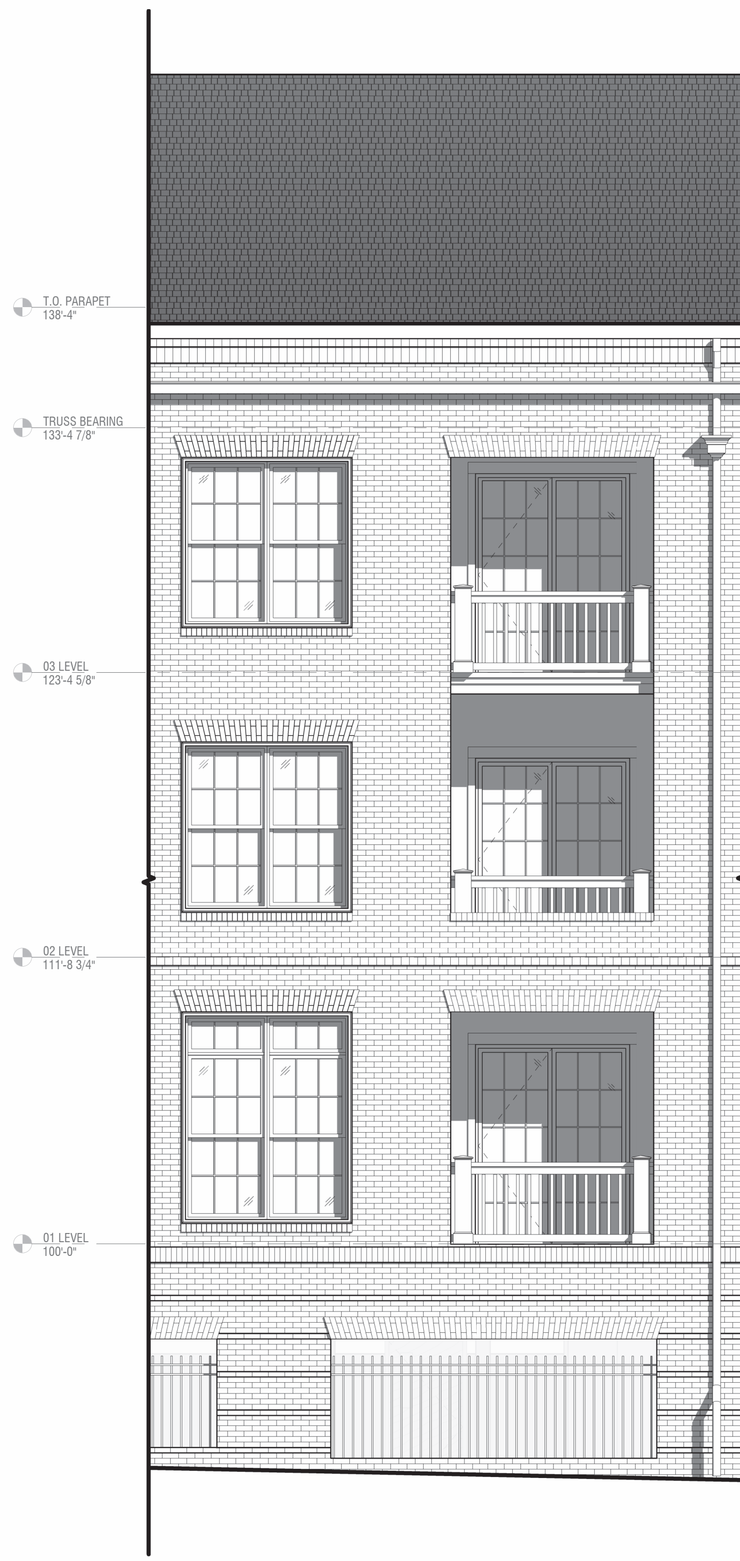
NORTH BALCONY ELEVATION 2 BUILDING ELEVATION SCALE 1/4" = 1'-0"
