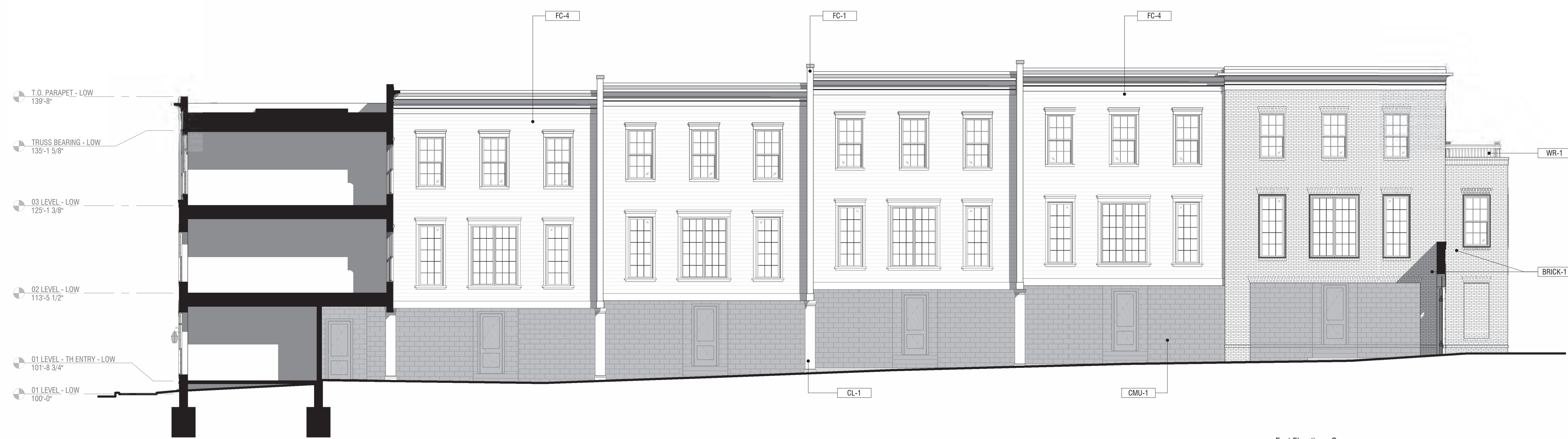
East Elevation - Garage 2 BUILDING ELEVATION SCALE 1/8" = 1'-0"
