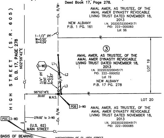
BASIS OF BEARING: The bearings shown on this plot were transferred from a field traverse originating and is based on the Ohio State Plane Coordinate System, South Zone as per NAD 83, 1986 adjustment. A bearing of North 10'31'41" East was held for a portion of the existing centerline of Reynoldsburg-New Albany Road, between centerline monuments FCGS 9916A and FCGS 9916B designated the "basis of bearing" for this plat.
