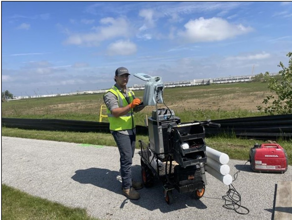
Tommy Diamond is conducting a CCTV Survey before construction begins at 9490 and 9500 Innovation Campus Way
