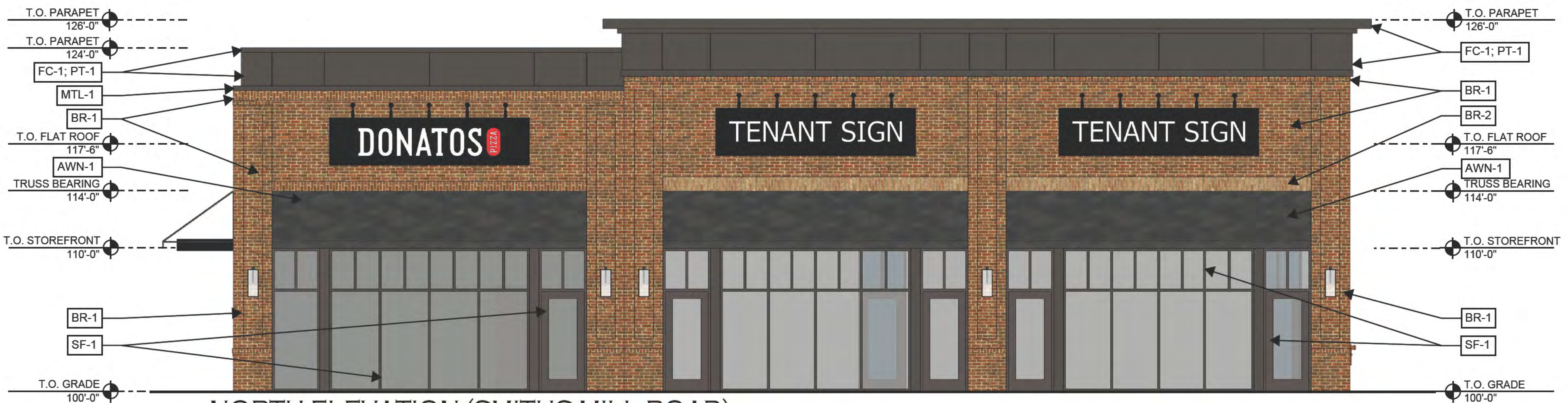
(A) NORTH ELEVATION (SMITHS MILL ROAD) SCALE: 3/32" = 1'-0"
