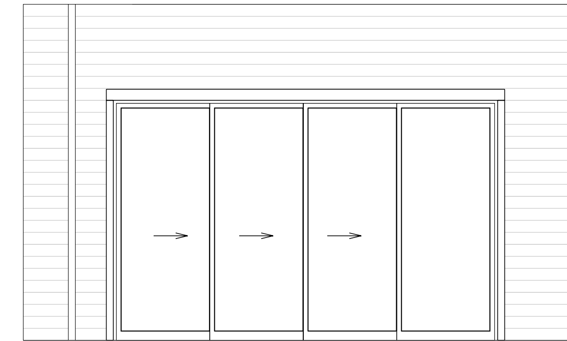
GREAT ROOM SLIDER ELEVATION SCALE: 1/4" = 1'-0"
