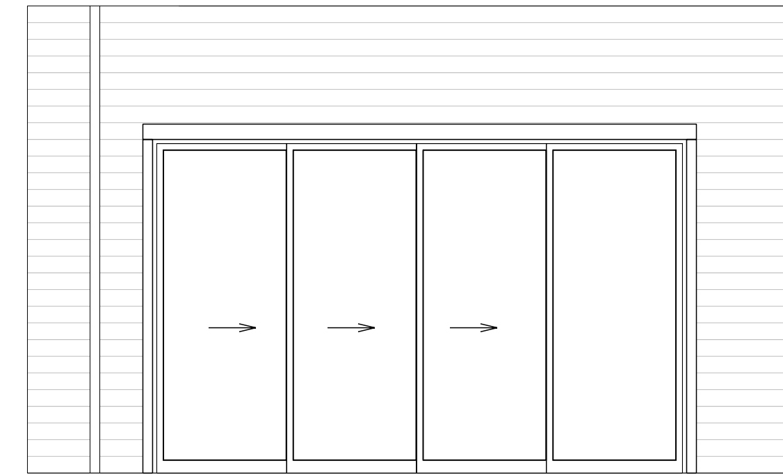
GREAT ROOM SLIDER ELEVATION SCALE: 1/4" = 1'-0"
