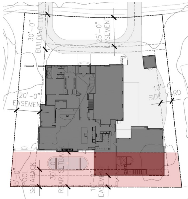
Image: Proposed site plan showing the approximate rear yard setback and encroachment in red.
